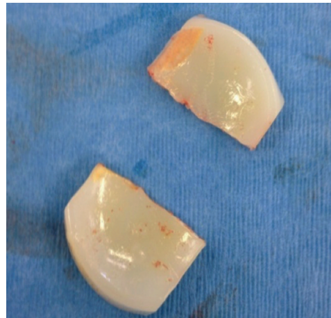
Fig. 2: Retrieved bearing insert showing the clean fracture through the thinnest part and minimal wear of the polyethylene insert.
