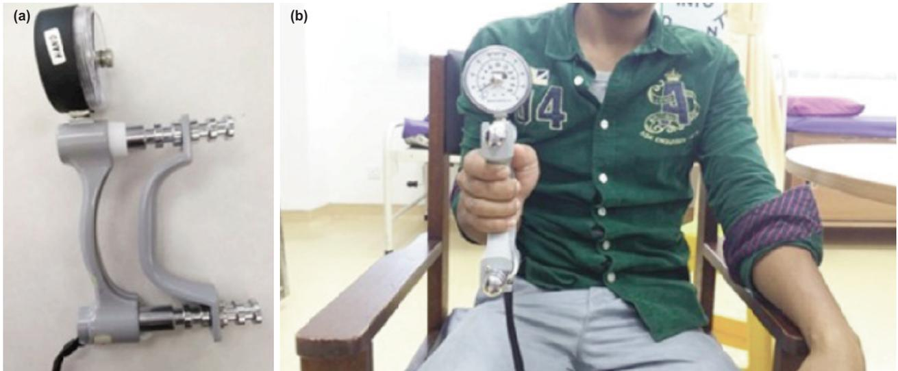
Fig. 2: (a) A photo showing a JAMAR hydraulic hand-held Dynamometer used in our study, (b) a photo demonstrating on how the measurement of grip strength was performed by using that device.
