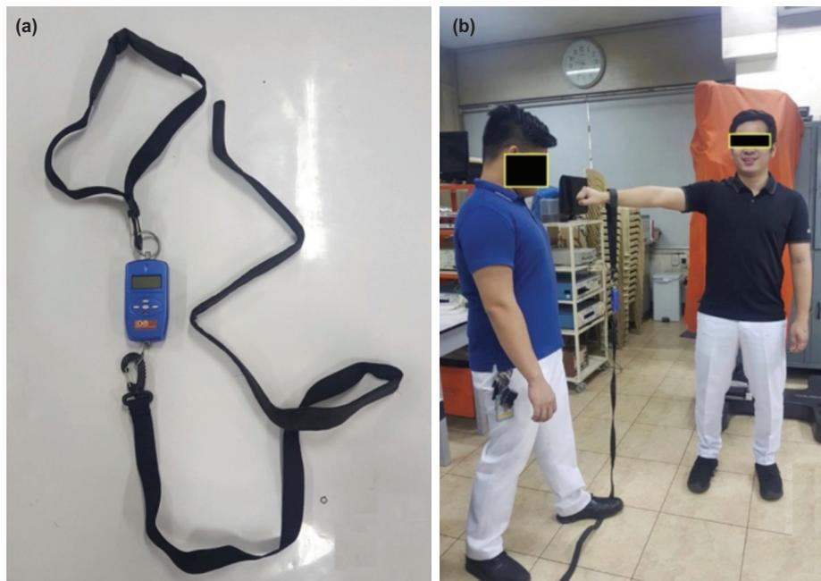
**Fig. 1:** (a) Handheld IDO isometer, (b) test position for participants.
