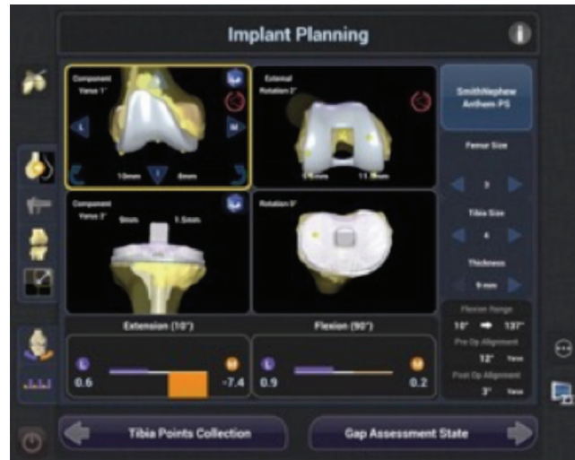
Fig. 1: Shows planning of external rotation of the femoral component as per mediolateral gap balancing in flexion and avoiding femoral notching (original photograph from robotic screen during surgery).
