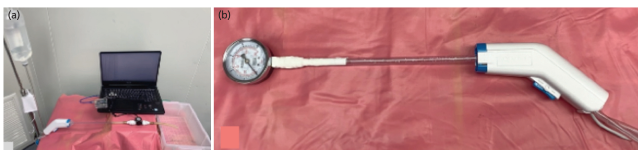
Fig. 4: (a) The flow rate and pulse frequency were measured through the water flow meter using a microcontroller board and program. (b) Analog pressure gauge was used for measuring the peak pressure of fluid ejection.
