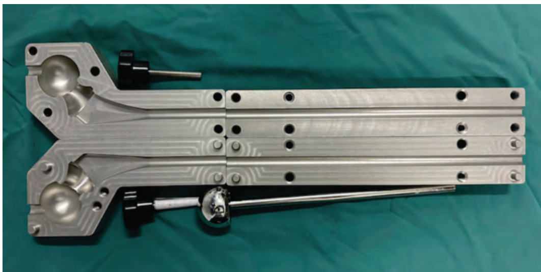
Fig. 2: The mold of the long femoral stem spacer.
