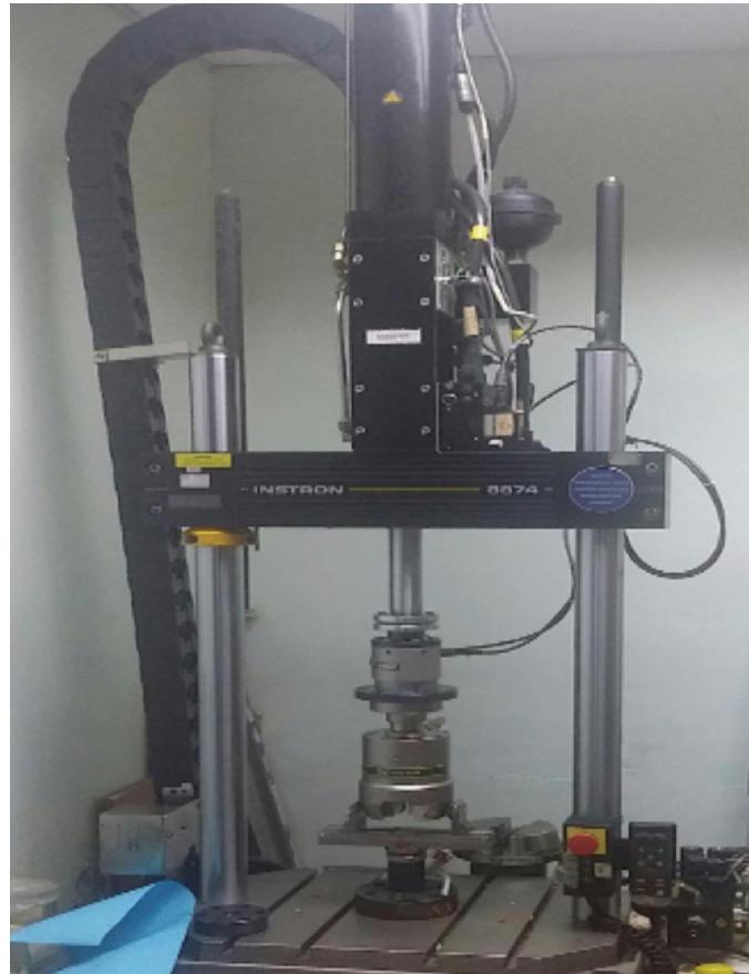
Fig. 2: 8874 Biaxial Servohydraulic Fatigue Testing, INSTRON [Illinois, USA] from Dental Laboratory, Universiti Sains Malaysia.
