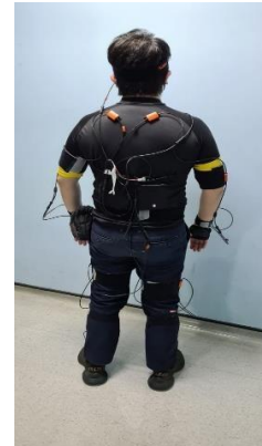
Figure 1: Showing sensor placement
