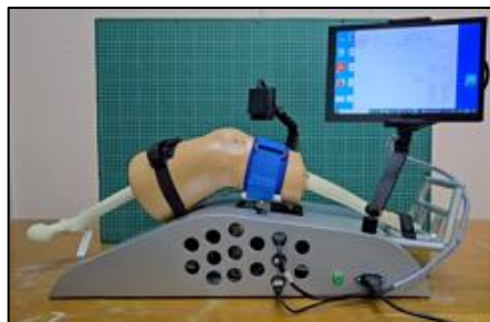
Figure 1. Prototype Lachman-O-Meter with synthetic knee model
